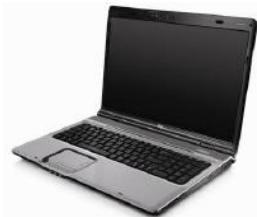
You can also buy a **laptop**, which is a small, light, compact computer which can easily be carried from place to place. Laptops combine the computer, monitor, and keyboard into a single unit, and they usually have a **touchpad** instead of a regular mouse.
