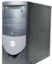
The **computer** is the box (sometimes called a **tower**) containing all the necessary parts and chips that make your computer operate, including the Central Processing Unit (or CPU), which is the brain of the computer.
